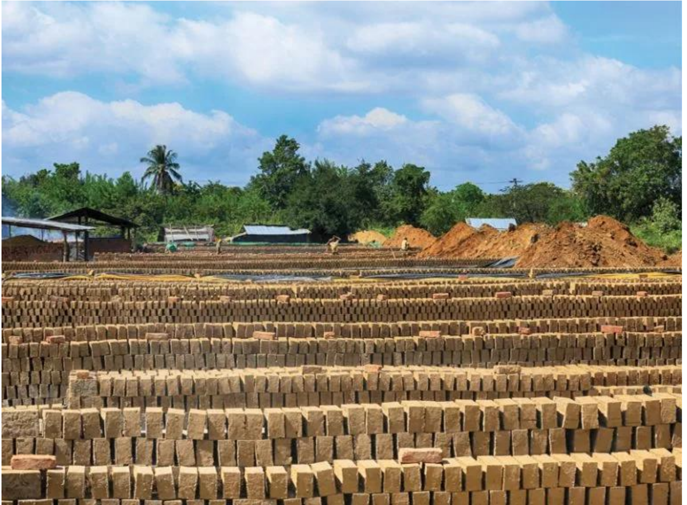
Rows of newly prepared bricks ready to be placed in the kiln
