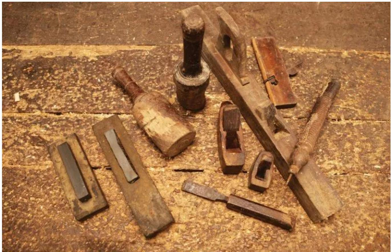
Now redundant tools like the oil stone, emery stone plainer, mallet, chisel, and driller
